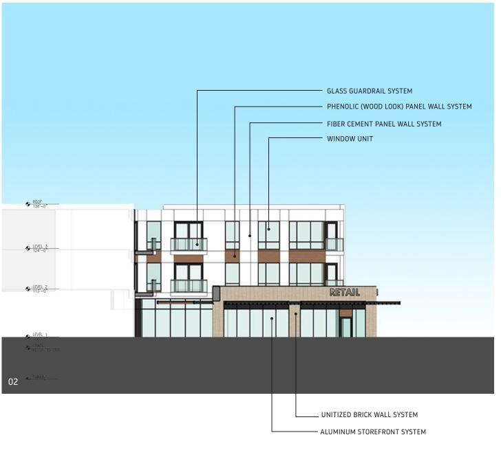
SOUTH ELEVATION - 01 NORTH ELEVATION - 01
