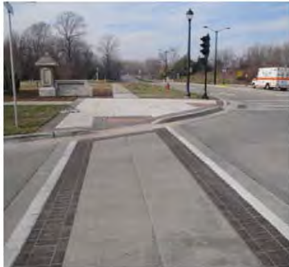
Concrete with brick paver border used for major intersection types. Painted stripes used for all other intersection types.
